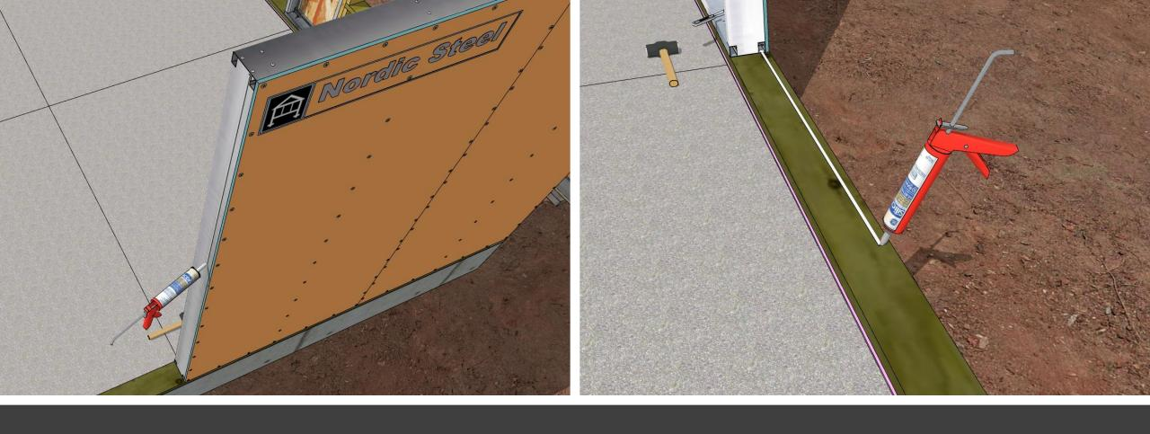
As with the previous panel, apply a bead of 100% Silicone to sill plate and edge of SuperPanel no more than 1" from outside edges.
