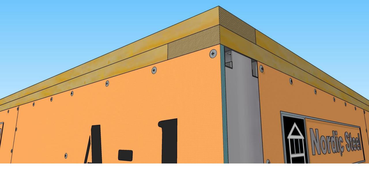
Twin, overlapping 2 x 6" Cap Plates are attached as soon as a corner is established and no less than 16' of wall erected. The first row of Cap Plates overlaps the corner, panel joint.
