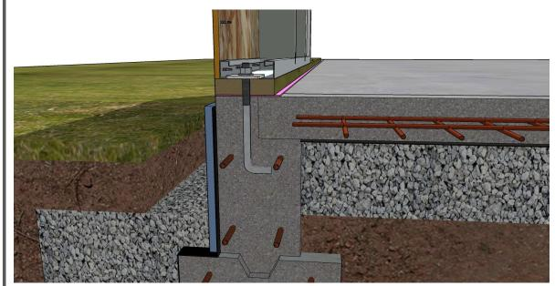
Anchor Bolts need to be embedded into concrete, 3 ¼" from outside edge at code required intervals. To accurately transfer the sill and SuperPanel hole locations, use a reliable speed square to transfer their location.
