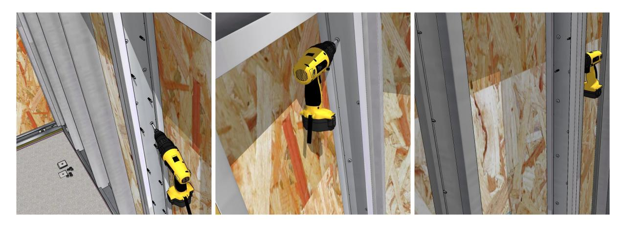
Fasten SuperPanels together with 2 staggered rows of screws, one on each opposite side set 2" apart and @ 8" OC.
