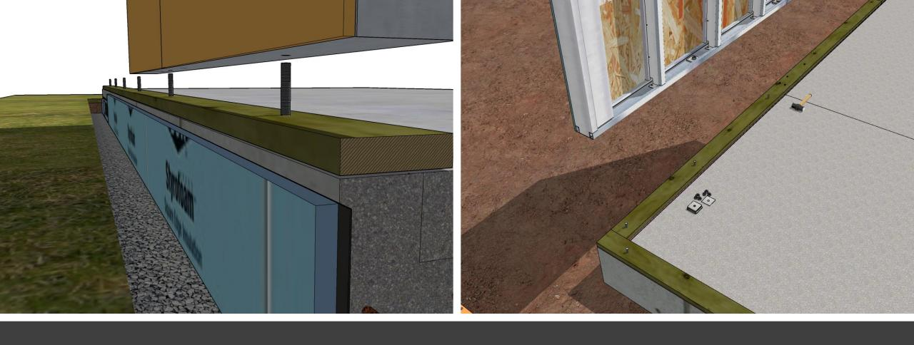
Lower SuperPanel onto anchor bolts and sill plate.
