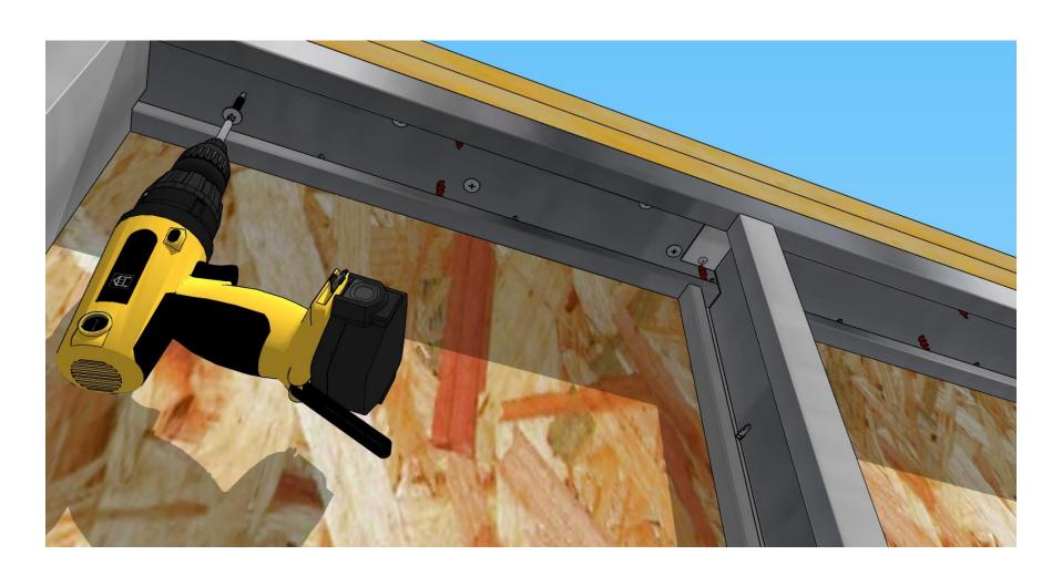
Once bottom Cap Plate row is affixed, run Timberloc screws or similar self tapping, 4" screws through top Cap Plate and into SuperPanel.
