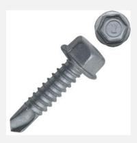
Each SuperPanel™ is fastened to the other by counter faced, staggered rows of self drilling, steel screws. Each row is set @ 16" On Center, staggered to achieve a fastening distance of 8" On Center from opposing sides.
