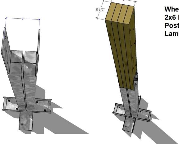
When Used with a 6" x 5 1/2", 4 Ply 2x6 Engineered Post, the Steel Post Halves Must Compress the Laminations of Engineered Post.
